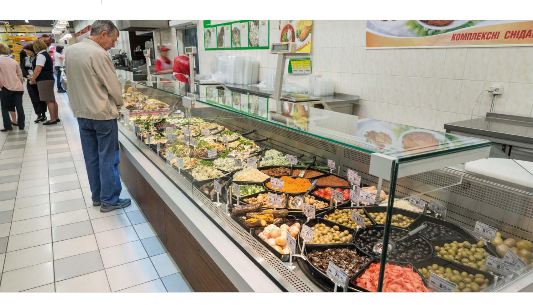
Island of refrigerated counters Cube with corner trapezoidal elements is equipped with an extra shelf for the convenience of customers – they can put there a bag or a basket with products. Counters are connected to remote cooling system, which is installed in the window of trading hall in sound- and heat-insulated casing
